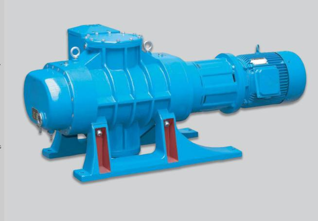
Airtech AC Series vacuum boosters are positive displacement, **magnetic drive**, and roots-type blowers intended for use in conjunction with a mechanical backing pump. The AC booster pumps have a simple weighted bypass design that allows start-up from atmosphere.
